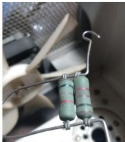
Another poorly built parasitic suppressor
