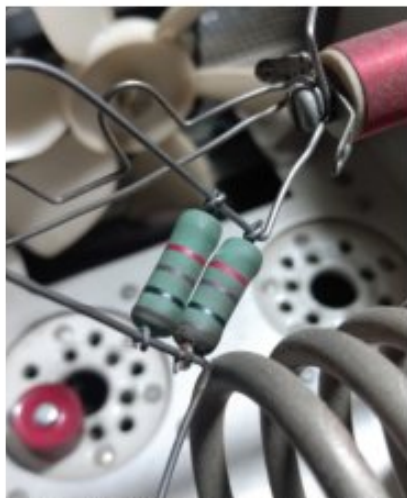
Poorly built parasitic suppressor
