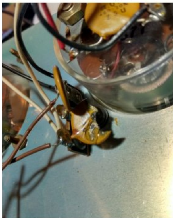
Blown capacitor on meter lamp circuit
