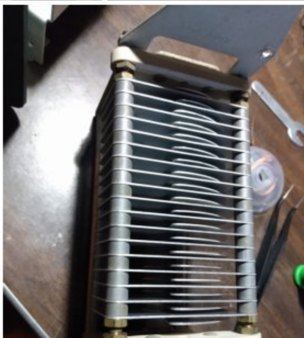
Repaired plate tuning capacitor
