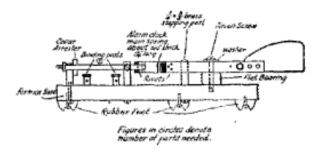
used on a "fast" bonus wire by myseif for a period of about 6 months, and by several other operators on faster circuits. The main reason for this peculiar looking piece of machinery is the defeat of cost. I am at present using the bug at 80T and can
