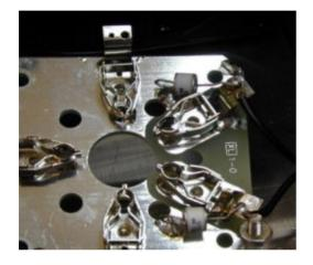
Completing Tom's list of mods, the final task involved the tube filament circuit: Removing Existing MOVs (Varistors) and Installing GDTs (Gas Discharge Tubes). These GDTs provide updated protection against dramatic tube failures. The process required removing the tube socket (which is essentially a bolted-in circuit board) and soldering in the GDTs. The existing MOVs were somewhat buried behind heat/RF shielding but were easily identifiable. With a bit of effort, they were snipped and removed.
