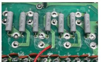
breeze. Simultaneously, I replaced the bleeder resistors—a surprisingly simple and straightforward task.
