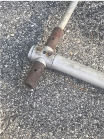
There is another element without traps that might be used for a single band rotatable dipole, it too is insulated from the boom.(2 Pictures below)
