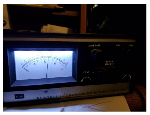
My CDE rotor control unit blew a bulb that lit the meter. Did a search for a led replacement. Bought one that had 6 small white LED's on a strip ready to solder across the old bulb socket. A little work and it ended up looking like a new piece of equipment. HI HI
